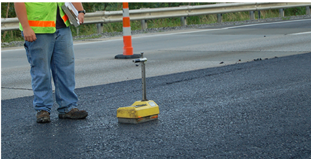
Asphalt compaction tests being conducted
